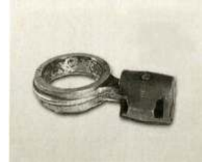
The lubrite coating on piston has been worn off
